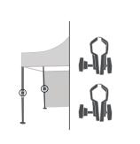
Take two of the Black Clamps and clamp one around the back Frame Leg, just above the Leg Adjustment Joint. Do the same to the adjacent front leg.
