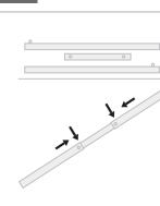
The Side Skirt Rail should be in three pieces. Slide the smaller rail into the larger rail to create one long rail.
