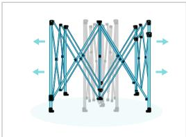
Grab one leg of the frame with each hand and lift up and out to extend the frame until it is near halfway open.
