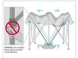
Grab the center cross bars with both hands and lift up until the frame is fully extended.
