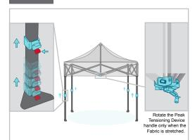
Go to each leg, place your foot on the canopy footpad, grab the leg and lift up to raise the canopy. Do this on all four corners until desired height is reached. Use the Peak Tensioning Device to raise canopy top.
