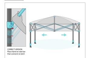
With one hand holding the frame leg, reach under the canopy top with the other hand, and push up until you feel it click into place. Do this on all four corners.
