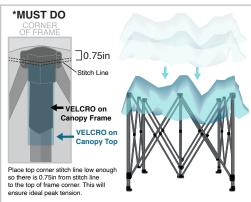
Place the canopy top over the frame. Go to each corner and attach the velcro inside the canopy top to the velcro on the top edge of the canopy frame.
